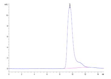
The purity of Mouse Fc gamma RIIB is greater than 95% as determined by SEC-HPLC.
